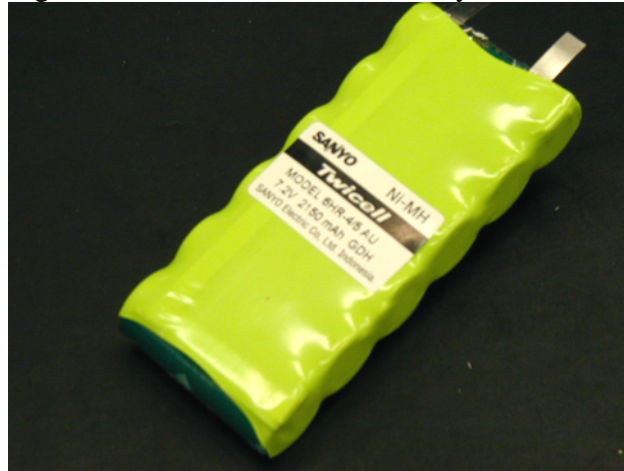
Figure 1 : TOPB5XX NiMH battery Pack
