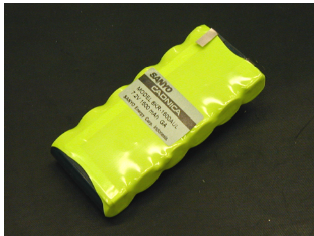
Figure 2: TOPB2XX NiCd battery pack.
